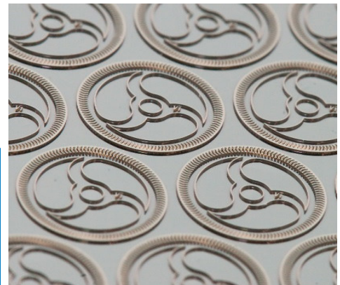
Micro gear. 200 \mu\text{m} high.
