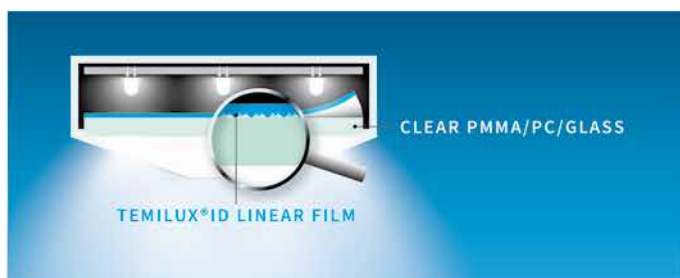
temilux®ID linear film with microstructures facing away from LEDs (inside)
