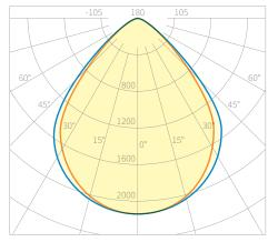
Measured\* light distribution curve of temilux®ID — C0/C180 — C90/C270
